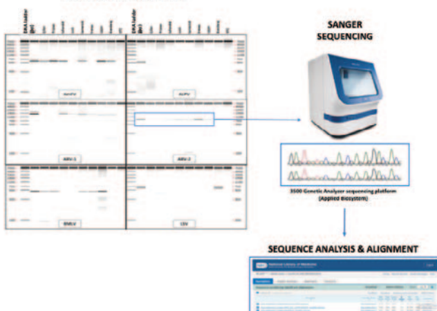
Figure 2. Capillary electrophoresis on LabChip GX Touch HT* of the PCR products for the six emerging honey bee viruses (AmFV, ALPV, ARV-1, ARV-2, BMLV and LSV). DNA ladder: from 100 to 7000 bp; PC: PCR positive control; NTC: PCR negative control. On the lower right, the results of alignment of ARV-2 sequences with those available in the GenBank database using BLAST.
